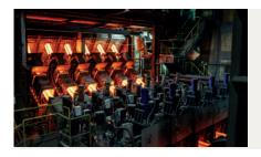
A continuous update of manufacturing **facilities**: recent investment in the **continuous casting machine for billets of 240x240 mm**, equipped with the latest control technologies.
