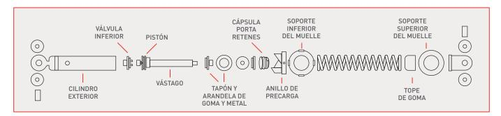
Conventional tourism shock absorbers are composed of various parts, among which the rod is an essential operational element. It is a cylindrical, cut-to-size and chromed part, which is made of special steel rods with guaranteed mechanical properties and high surface quality for easier subsequent chrome-plating.
