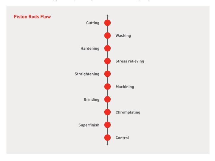
The material used to manufacture this component is an elongated or elongated + turned SAE1040 with diameters between 15 and 30 mm, which shall ensure a minimum limit of elasticity of around 600 MPa.
