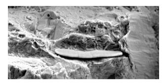
The elongated shape of MnS deteriorates the steel isotropy, negatively affecting the transversal properties
