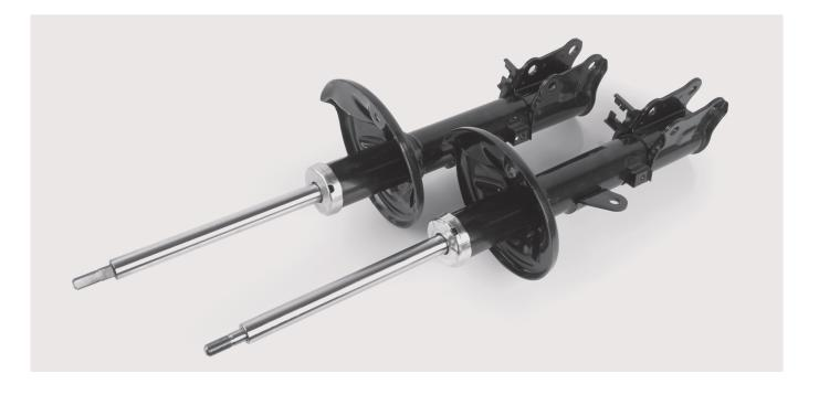
To conclude, both qualities presented by Sidenor meet the needs of the shock absorber rod, while providing cost savings related to the elimination of induction hardening.
