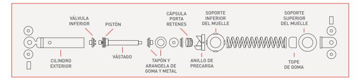
Conventional tourism shock absorbers are composed of various parts, among which the rod is an essential operational element. It is a cylindrical, cut-to-size and chromed part, which is made of special steel rods with guaranteed mechanical properties and high surface quality for easier subsequent chrome-plating.
