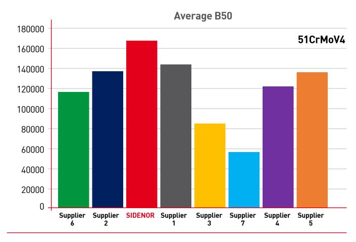
Benchmark of leaf spring steel suppliers by component fatigue testing at customer facilities
