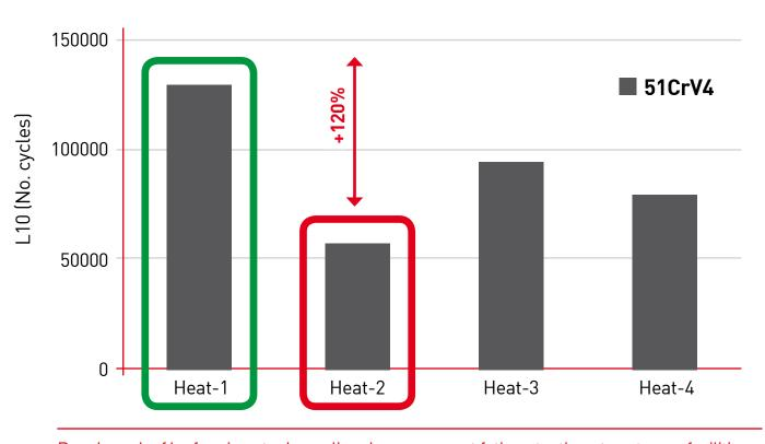
Benchmark of leaf spring steel suppliers by component fatigue testing at customer facilities
