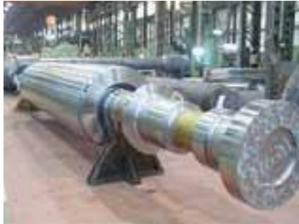
Generator rotor shaft
