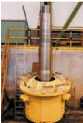
Rudder stock assembly (with steering gear)
