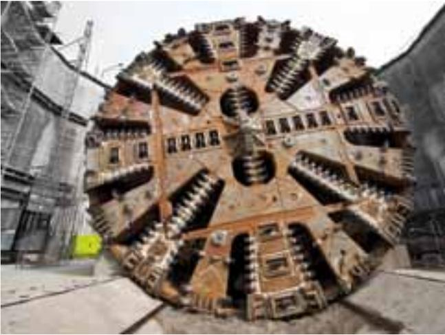
**Components for Tunnel boring machines**
