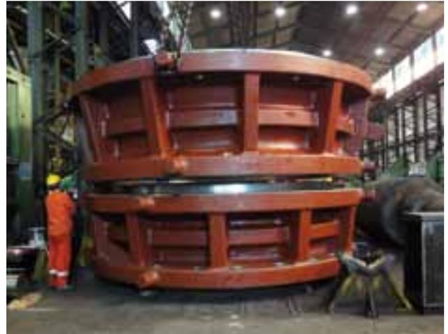
**Gyratory crusher (stack test)**
