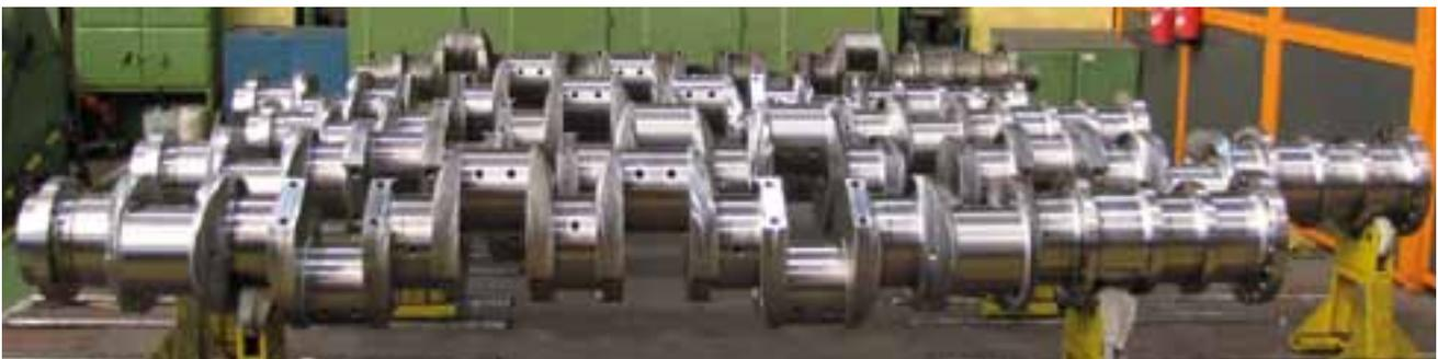
**Crankshafts for compressors**
