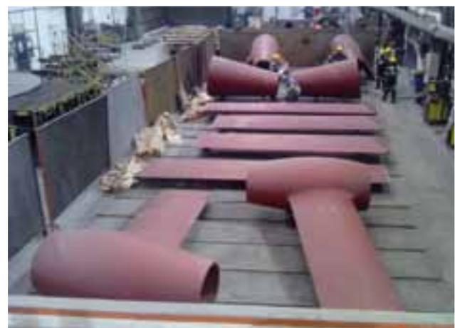
Boss piece, inner and outer bracket and shaft bearing
