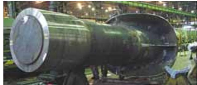
Complete assembly stern tube for LNG
