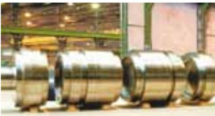
Modules/Discs gas-steam turbine shafts
