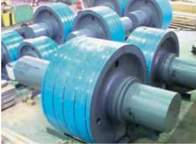
**Assembly of roller & roller shaft**
