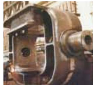
**Main casting for mooring system offshore**
