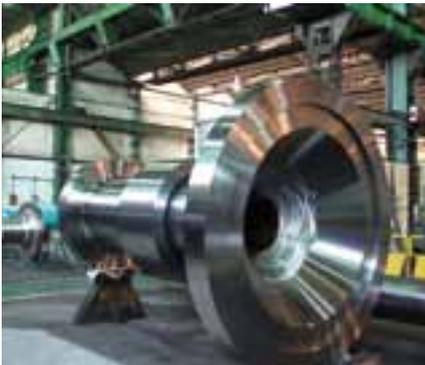
Hydro generator shaft (Ø 2400 mm)
