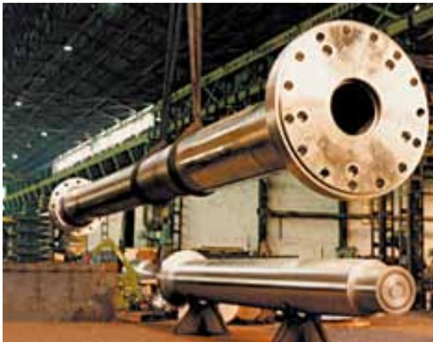
Propeller and intermediate shaft
