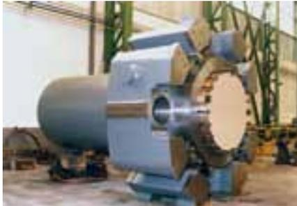
Cylinder for extrusion press
