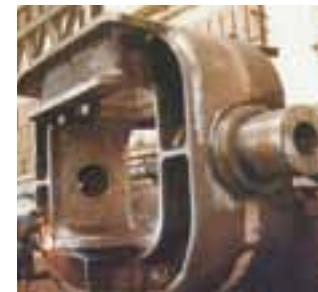
Main casting for mooring system offshore
