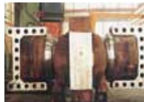
Main casting for mooring system offshore
