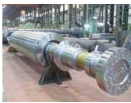
Generator rotor shaft
