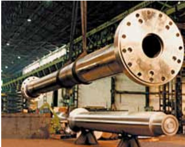
Propeller and intermediate shaft
