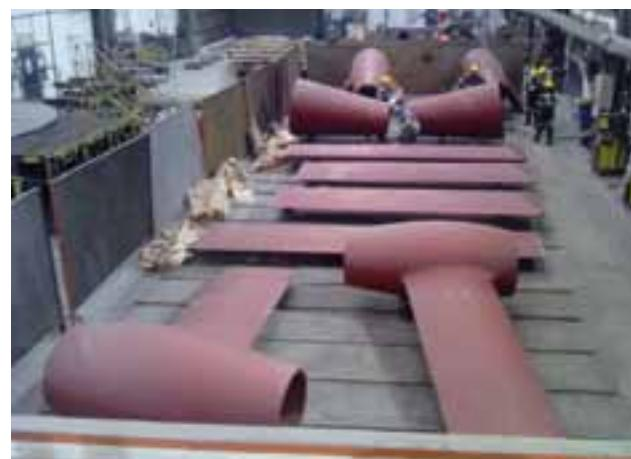
Boss piece, inner and outer bracket and shaft bearing
