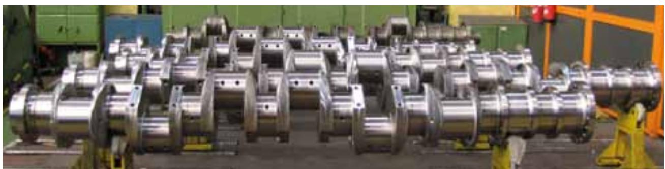
**Crankshafts for compressors**
