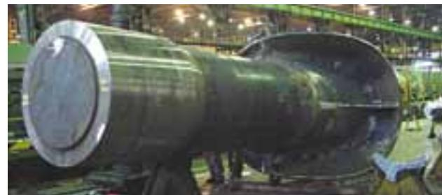
Complete assembly stern tube for LNG
