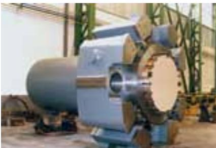
**Cylinder for extrusion press**
