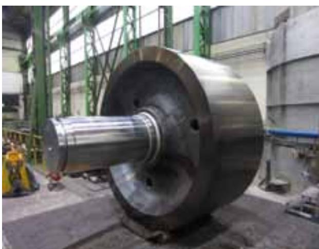
Assembly of roller & roller shaft
