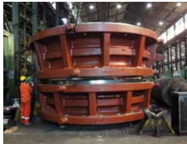
Gyratory crusher (stack test)
